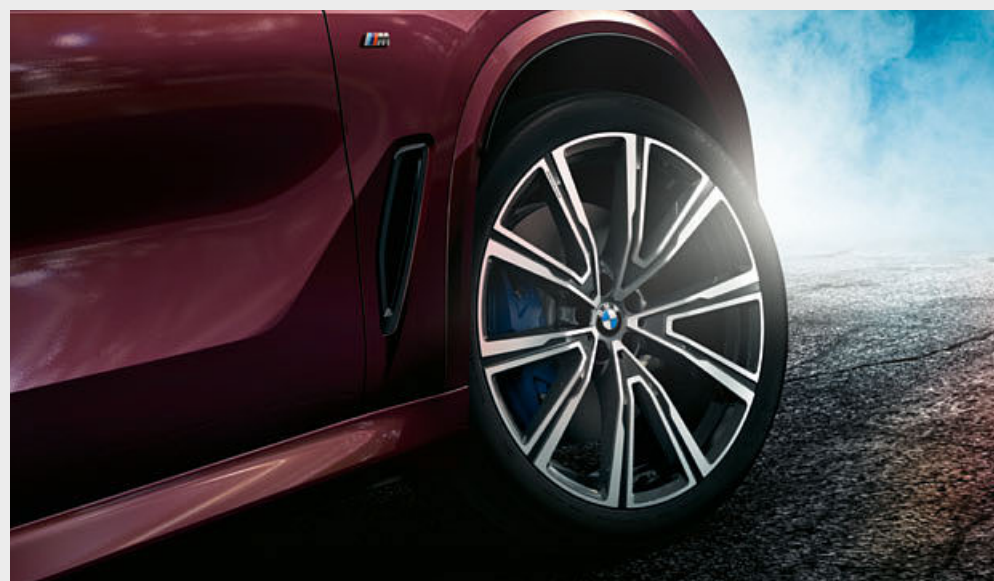
□ 22" BMW Individual light alloy wheels V-spoke style 746 I Orbit Grey with mixed tyres, burnished, front 9.5J x 22 with 275/35 R22 tyres, rear 10.5J x 22 with 315/30 R22 tyres.
