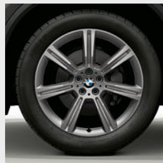
□ 20" light alloy wheels Star-spoke style 736 Ferric Grey with mixed tyres and runflat tyres, front 9J x 20 with 275/45 R20 tyres, rear 10.5J x 20 with 305/40 R20 tyres. 5,6
