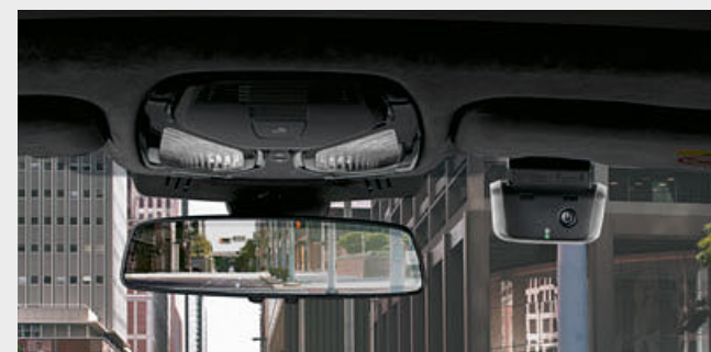
○ The BMW Advanced Car Eye 2.0 is a highly sensitive full-HD camera that captures events in front of and behind the car, even when it is parked. In the event of disturbances and extraordinary movement outside the vehicle, the camera automatically records the situation in order to document possible accidents or (attempted) break-ins.
