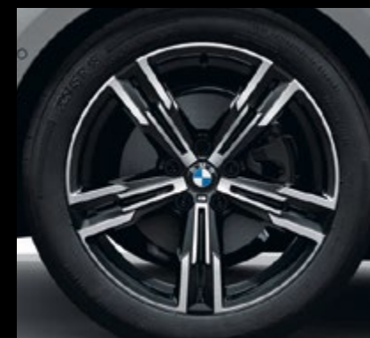
18" M light alloy wheels Double-spoke style 848 M Bicolour Jet Black with mixed tyres, gloss-lathed, wheel size front 7.5J x 18 with 225/45 R18 tyres, wheel size rear 8.5J x 18 with 255/40 R18 tyres. 1
