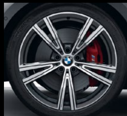
19" BMW Individual light alloy wheels Double-spoke style 793 I Bicolour Orbit Grey with mixed tyres and run-flat tyres, gloss-lathed, wheel size front 8J x 19 with 225/40 R19 tyres, wheel size rear 8.5J x 19 with 255/35 R19 tyres.
